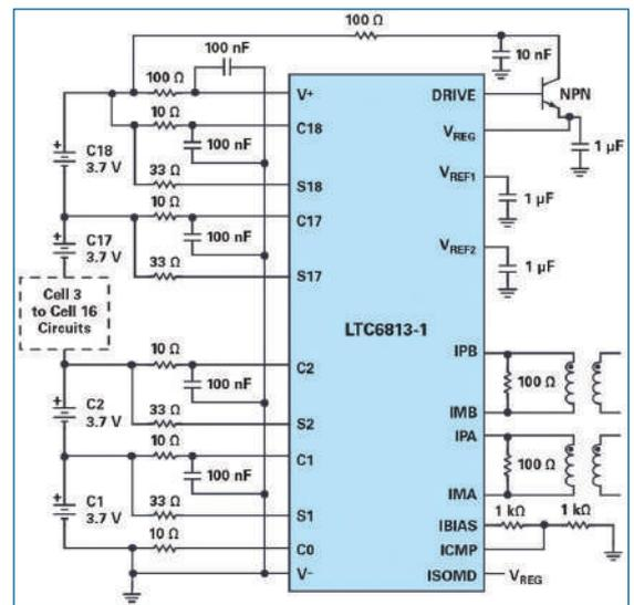
Fig. 3: LTC6813 application schematic.
