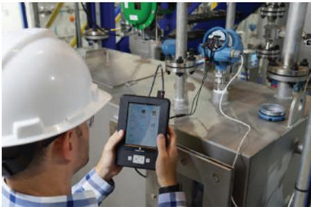
Emerson has added the Radar Master app for the AMS Trex device communicator, making it easier for field technicians to safely and efficiently configure Rosemount radar level transmitters. Radar level devices are critical to help deliver accurate, reliable measurements on both liquid and solid materials. The new app allows users to easily bring the radar configuration tools of Radar Master software to the field. Radar level devices in the field are typically mounted in
