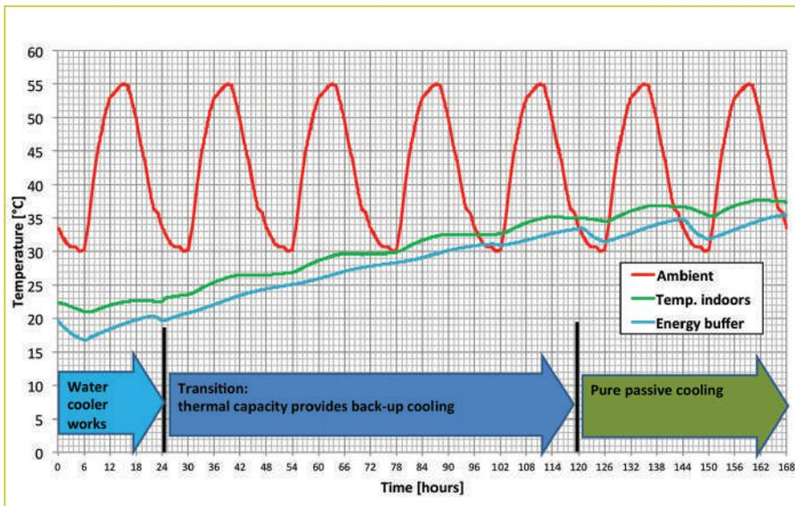
Fig. 2: Passive cooling can handle electricity outages or failure of powered cooling elements, as this one-week graph illustrates. This shelter's passive cooler was sized to maintain internal air temperature below 40°C, even if ambient temperatures reach 55°C – a worst case for its Mid-East location.
