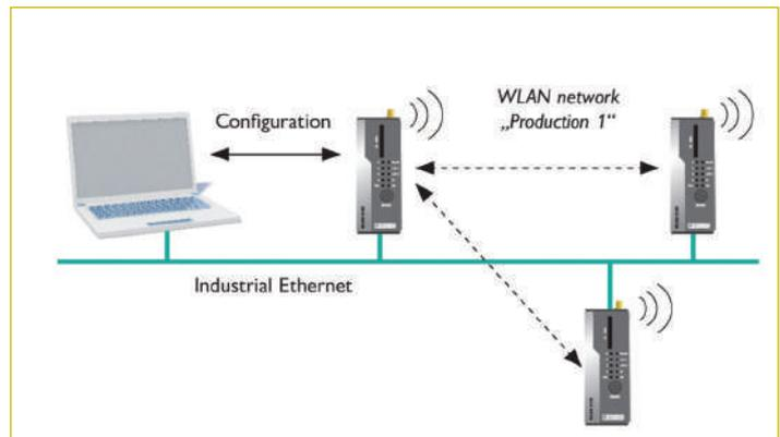
Fig. 3: Process control teams can quickly and easily set up a WiFi network in the production environment using cluster management technology. All access points can be configured collectively via a web interface.
