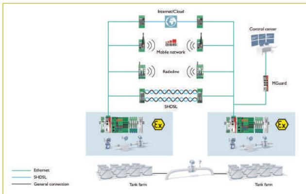
Fig. 2: The SHDSL modulation method enables existing cables to be used to transmit Ethernet or fieldbus signals. This allows for hybrid solutions in which the wireless network is used only for some signals.
