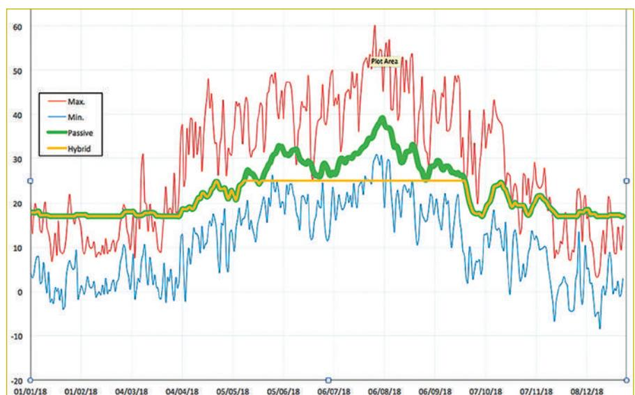
Fig. 1: Active and passive cooling elements working together over a year. Red and blue traces show daily min/max temperatures. Yellow shows normal hybrid operation with passive cooling boosted by active cooling in hot months. Green shows emergency mode, with passive cooling only.
