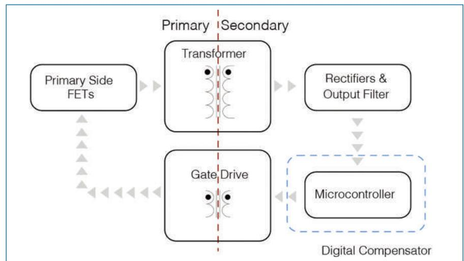
Fig. 2: A digital controlled power supply
