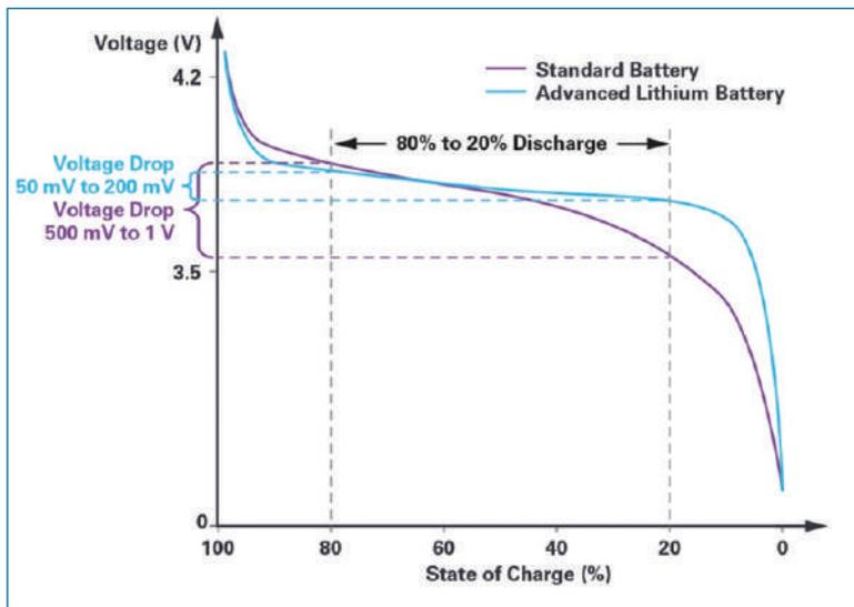
Fig. 2: Lithium battery discharge profile
