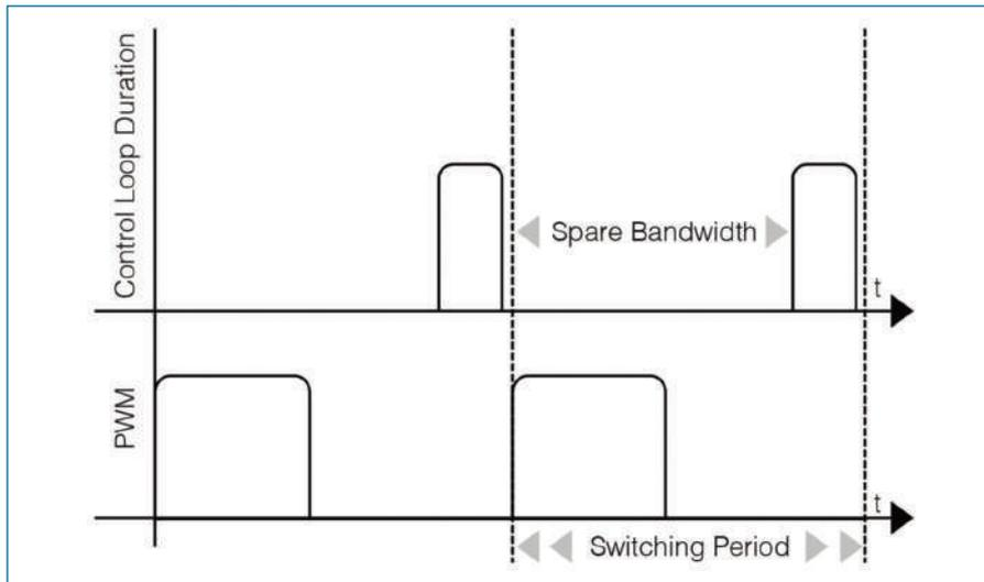
Fig. 3: Typical control loop duration vs PWM switching period
